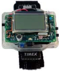
Figure 2 A sensor designed to appear like a common watch as used in the eWatch system [8]
