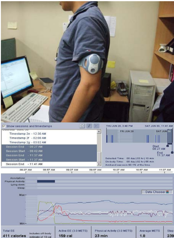
Fig. 1. The Armband worn on the left upper arm (top) and the screen of Innerview professional 5.0 (bottom)
