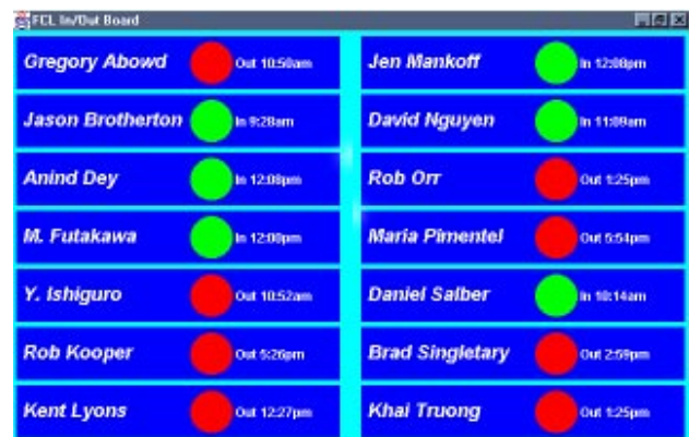
Figure 1. Screenshot of the in/out board application. The dot next to a user name is green if the user is in and red if she is out.
