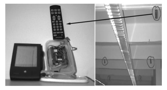
Figure 3: IR positioning prototype (left) and the array of positioning beacons in the GVU Lab (right).
