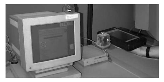
Figure 7: Home-made ir units allow cross-platform communication.
